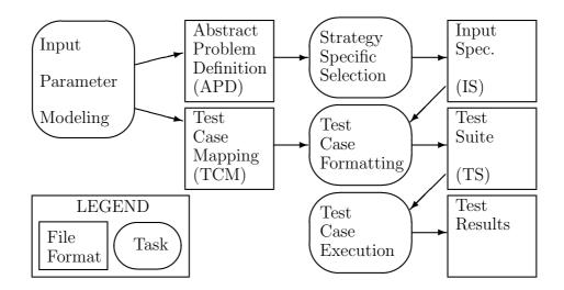
Figure 5: Test Case Generation and Execution
